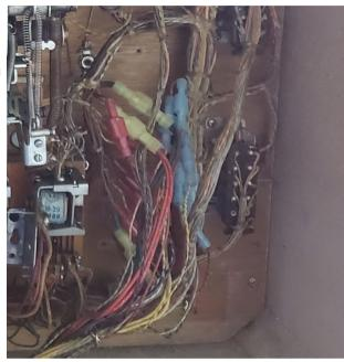
Above you can see an example of mistreatment. For whatever reason the 24 pin connector here was just ripped out. We replaced these with quick disconnect crimps. Not as convenient, but a lot easier than fabricating a 24 pin connector. You can see the smaller original ones right of center. Moral of the story, don't let drunk people work on relay logic machines.
